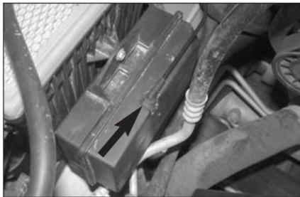
4. Disconnect the vacuum canister hose shown.
