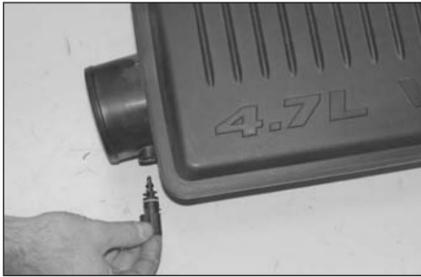
24. Rotate the air temperature sensor counter clockwise and remove the sensor from the stock intake plenum as shown.
