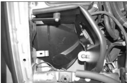
19. Install the heat shield assembly into the vehicle and secure it to the mounting locations with the provided hardware.
