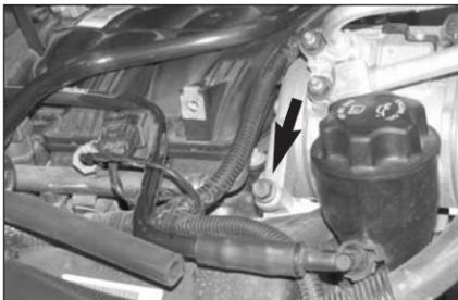
22. Remove the lower rear A/C mounting bolt shown.
