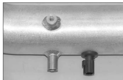
27. Install the air temperature sensor into the K&N intake tube as shown.
