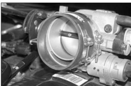
21. Install the silicone hose (084031) onto the throttle body and secure with the provided hose clamp.
