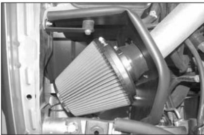
34. Install the air filter assembly onto the K&N intake tube as shown and secure with the provided hose clamp.
