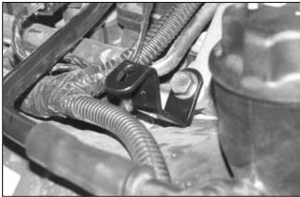
23. Install the tube mounting bracket onto the A/C compressor and secure with the factory mounting bolt removed in step #22.
