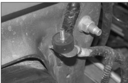
18. Install the 6mm male/male rubber mounted stud onto the upper air box mount as shown.
