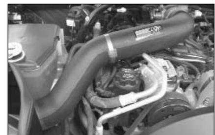
29. Install the K&N intake tube into the silicone hose at the throttle body and onto the saddle clamp, then secure with the provided hose clamps as shown.
