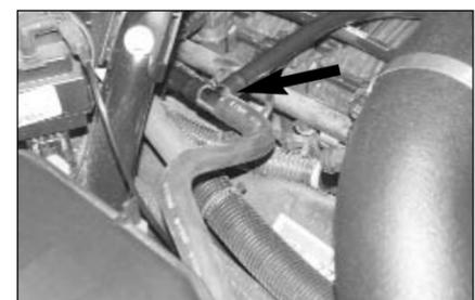
30. Remove the factory crank case vent hose from the "T" fitting shown.
