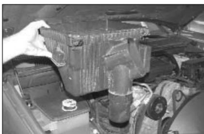
9. Lift the lower air box and remove it from the vehicle as shown.
