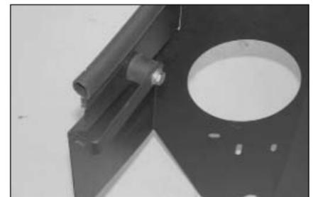
12. Install the bracket/rubber mounted stud assembly onto the heat shield as shown using the provided hardware.
