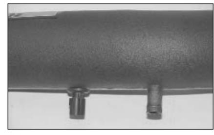
28. Install the air temperature sensor into the K&N intake tube as shown.
