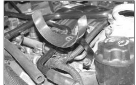
24. Install the tube mounting bracket assembly onto the A/C compressor and secure with the factory-mounting bolt removed in step #23.
