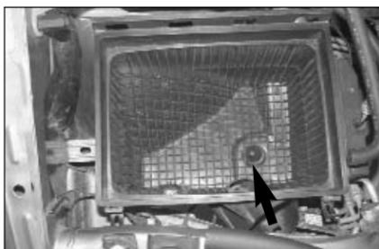
8. Remove the air box mounting bolt shown.
