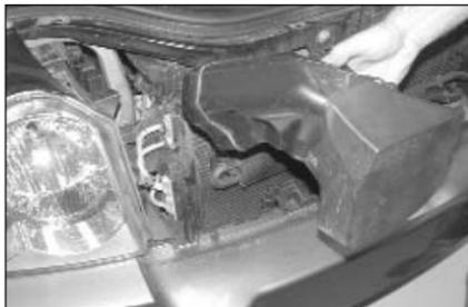
7. Pull the fresh air duct forward to disconnect it from the air box and then remove it from the vehicle.
