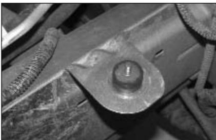
17. Using the two fender washers and one rubber washer, install the 6mm male/female rubber mounted stud onto the lower air box mount as shown.
