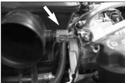
20a. Disconnect the air temperature electrical connection.
