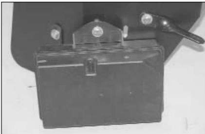
15. Using the provided spacer, install the vacuum reservoir onto the heat shield as shown.
