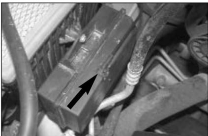
4. Disconnect the vacuum canister hose shown.
