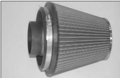
32. Install the filter adapter into the air filter as shown, secure with the provided hose clamp.
