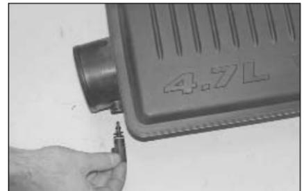
25. Rotate the air temperature sensor counter clockwise and remove the sensor from the stock intake plenum as shown.
