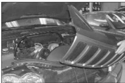
6. Remove the six grill retaining clips from the grill, then tilt the grill forward and lift to remove from the vehicle.
