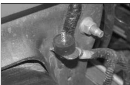
18. Install the 6mm male/male rubber mounted stud onto the upper air box mount as shown.
