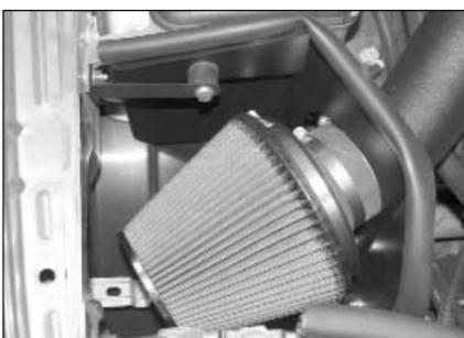
34. Install the air filter assembly onto the K&N intake tube as shown and secure with the provided hose clamp.
