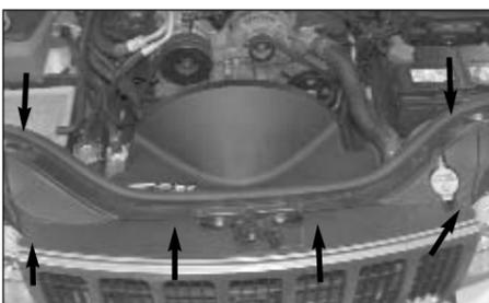
5. Using a small screwdriver, release the center holding pins in the six grill retaining clips shown.
