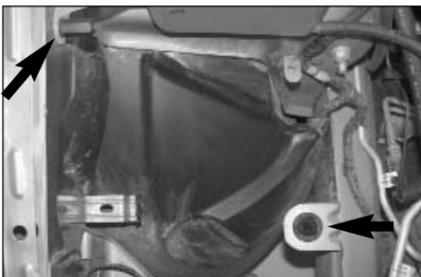
16. Remove the coolant reservoir-retaining nut and air box mounting grommet shown.
