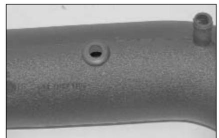
26. Install the supplied rubber grommet into the K&N intake tube as shown.
