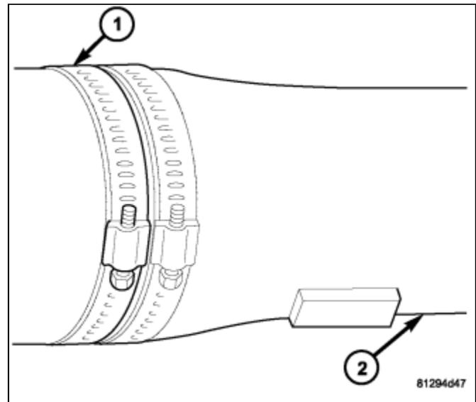
13. If the additional clamp causes an additional vibration, separate the first clamp (1) and second clamp (2) (1/4 inch above and below the mark). Repeat the vibration test.
