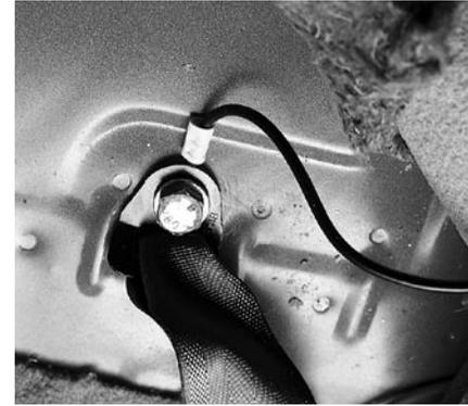
*Bolt the ground terminal tightly to the vehicle's metal chassis.*
