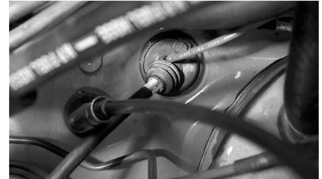
*Fuse installed on power wire, and secured in engine compartment.*
