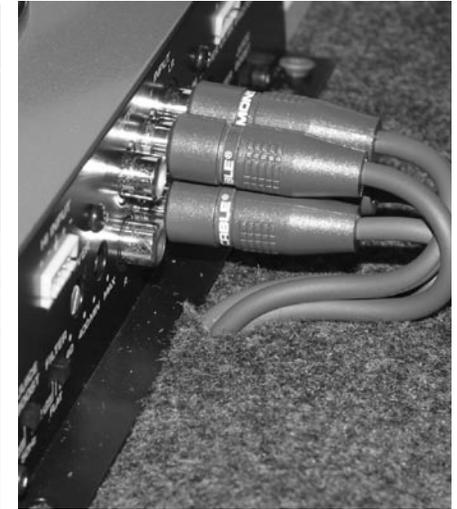
*RCA cables routed through slits in the vehicle's carpet, and connected to the amplifier's signal inputs.*
