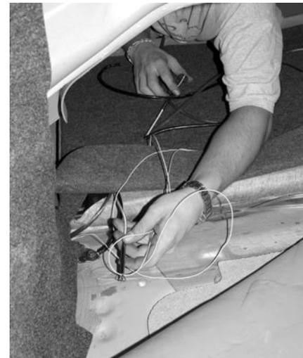
*A wiring snake can come in handy for pulling wires to the amp mounting location.*
