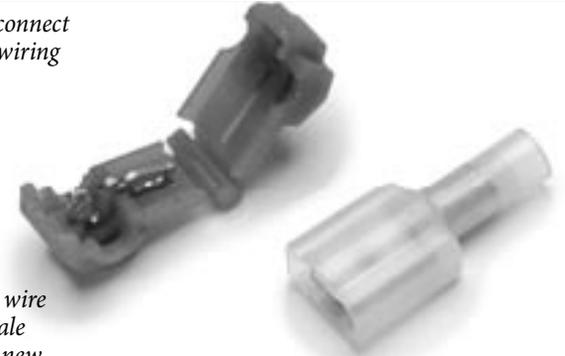
The male disconnect slides firmly onto the end of the wire tap, making a secure connection.
