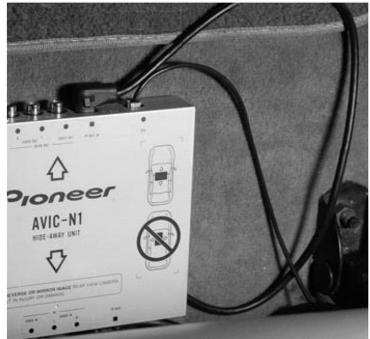
*All wires, including power, audio, and video, must be run from the navigation unit to the appropriate locations, usually under the vehicle's carpet.*
