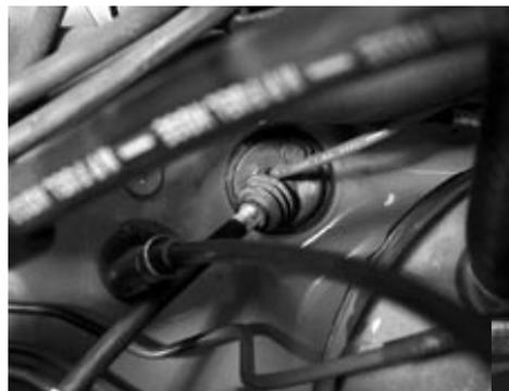
When running a wire from under the hood into the cab through the vehicle's firewall, we recommend you find and use a pre-existing opening, where other wires come into the vehicle cab.
