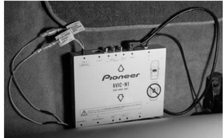
*The best place for the navigation unit itself is on the floor. For the gyroscope to work accurately, you must make sure the unit is mounted horizontally, and aligned correctly with respect to the vehicle. ("Brain box" of the Pioneer AVIC-N1 navigation receiver shown above.)*
